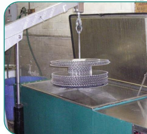
*Dirty blades go into the Omegasonics PowerPro 6000, still carefully stacked as they were during transport to the shop.*
