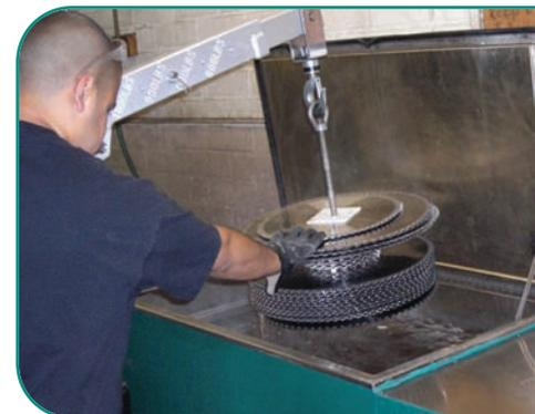
*After a two-minute cleaning cycle, the stack is lifted out of the Omegasonics and tilted to drain water from between the blades.*
